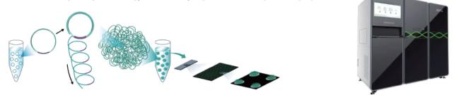
The combination of linear amplification and DNB technology reduces the error rate while enhancing the signal. The size of the DNB is controlled in such a way that only one DNB is bound per active site on the DNBSEQ flow cell. This densely patterned array technology provides optimal sequencing accuracy and increases flow cell utilization.
